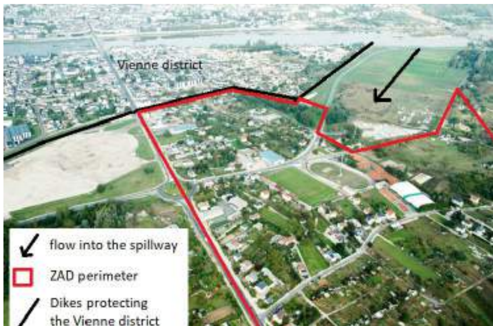
Figure 11. La Bouillie district, surrounded by the ZAD perimeter before the de-urbanization process.
